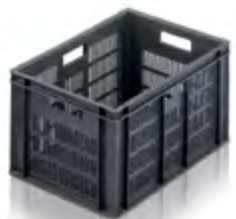
ES210601: 60 litres Ventilated Euro stacking Ext: 600 x 400 x 319mm Int: 555 x 355 x 294mm Wt: 2.33 Kg, Colour: grey
