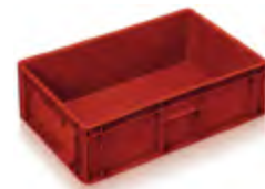
ES641704: 34 litres Solid Euro stacking Ext: 600 x 400 x 175mm Int: 556 x 356 x 162mm Wt: 1.8 Kg Colour: grey or red
